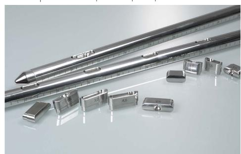
With the Novartos pharmaceutical samplers, multiple individual dose samples (unit dose samples) can be taken from one or more sampling points in a single sampling.
